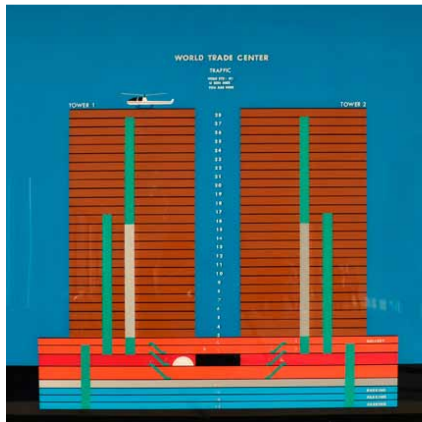
The conception of tower buildings as a vertical zoning plan, stacking parking, commercial base and office spaces.
